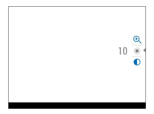
**Brightness** - press the **UP (5)/DOWN (3)** buttons to change display brightness from 0 to 20.
