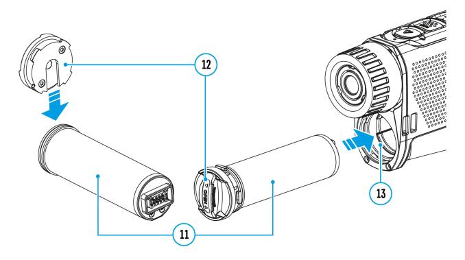
**Attention!** Before installing the battery, make sure that there is an undamaged rubber insulating ring on the battery. The ring is designed to protect your device from moisture getting inside. Damage to the device due to a missing ring is not covered by the warranty. To replace or purchase a ring, contact your **local distributor.**
