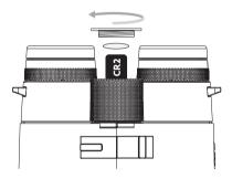
If there is no battery, insert it with the correct polarity (see the marking on the battery compartment cover). Turn the battery cover clockwise. At 20 °C the new battery is sufficient for approx. 2,500 measurements. However, depending on the conditions of use, e.g. in lower temperature or in case of more frequent use of the continuous measurement (scan) mode, the battery life can be significantly shorter. Be sure to check the battery indicator on the display.
