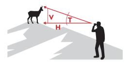
**T.** Angle measurement. This is the angle of the binoculars relative to the observed object.
