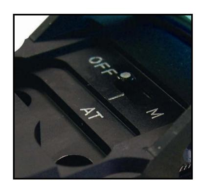
available with the use of the Photosensor. Please ensure you return the switch to the OFF position after use to avoid battery failure. Note replacing the cover does not turn the sight off.
