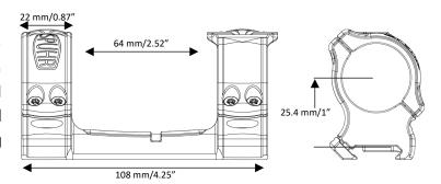
The SCP-3000D Interface Mount features two Spuhr Interface™ Top Covers, which can be installed as to position any of more than 40 different accessories in either the 12 or 3 o'clock position.
